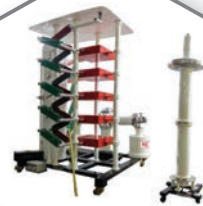
Impulse Generator up to 500 kV
