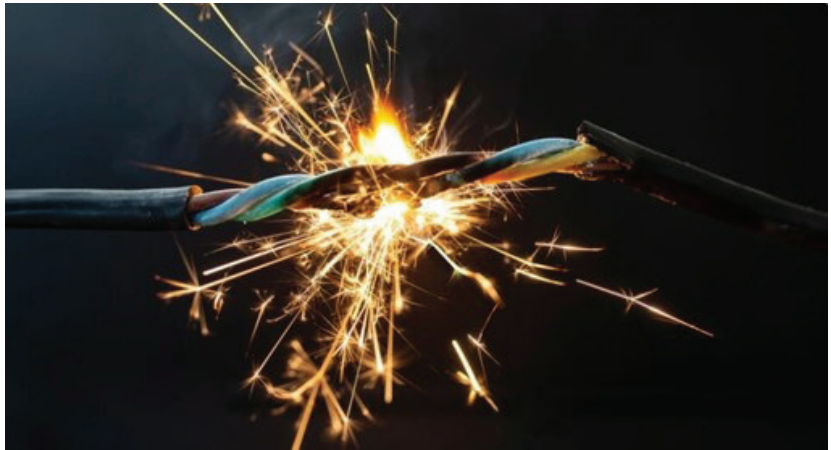
Fig 5: Fire due to Insulation Failure
